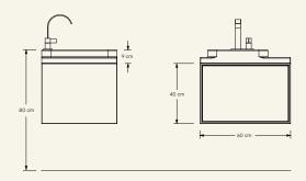
Name Kauai Designer Fábio Teixeira, 2017 Materials & finishings Sink in carved marble with honed matte finish and cabinet in wood veneer. Instalation wall-mounted Production details Washbasin obtained from a single piece of marble, CNC carved, and finished by hand. Dimensions (cm) H49 x L60 x D50 Weight (kg) approx 55
