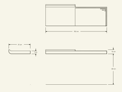
Name Bali Designer TCC Whitestone Industrial Design Studio, 2016 Materials & finishings Sink in carved marble with honed matte finish. Instalation wall-mounted Production details Washbasin obtained from a single piece of marble, CNC carved, and finished by hand. Dimensions (cm) H10 x L150 x D51 Weight (kg) approx 35
